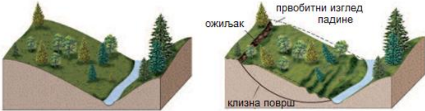
Figure 10. Slope slope caused by the intersection of the river flow [3]
