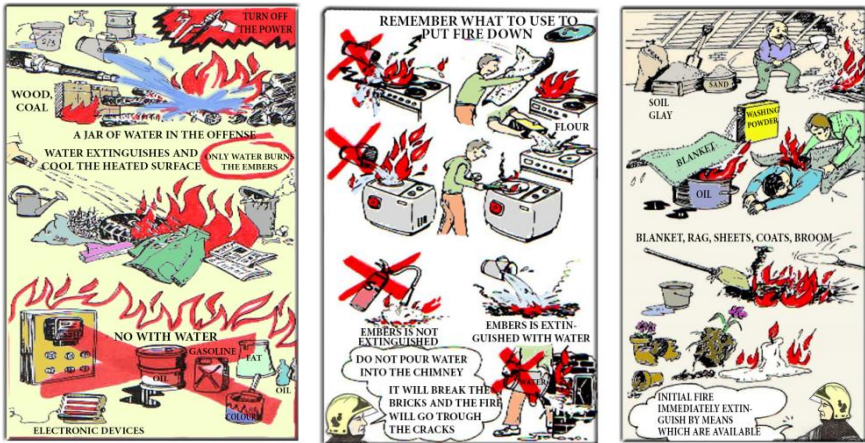
Figure 12. Basic rules and procedures for fire extinguishing (Source: Arnaudović, 2007).
