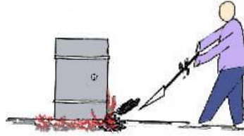
Figure 11. Covering the leaked burning fluid with the sand
