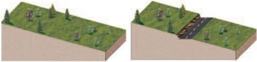
Figure 9. Sloping slope caused by slope cutting [3]
